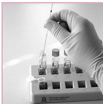
2. Transfer 20 µL of the sample (serum/plasma) with a ringmark capillary into each cuvette
