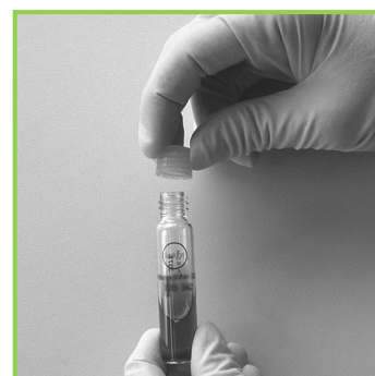
6. Replace screw cap with starter cap
