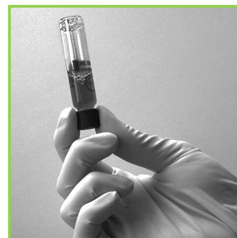
3. Screw cap on Turn cuvette upside down several times
