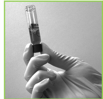
3. Screw cap on Turn cuvette upside down several times
