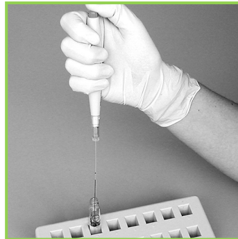
2. Eject sample several times with micropipetter into cuvette
