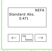
**6.** Insert cuvette 2 (standard) into photometer
