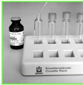
**3.** After a waiting time of 10 minutes, pipette 500 μL solution R2a from the bottle into each cuvette
