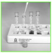
**2.** Pipette samples into cuvettes, mix well and leave them for 10 minutes
