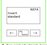
**5.** Zero point adjustment: Insert cuvette 1 (blank for zero point) into photometer
