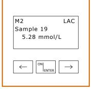
**9.** Insert the last cuvette, read the measured value, remove cuvette
