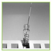
1. Insert capillary with 10 μL sample into cuvette
