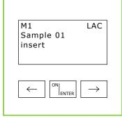
**4.** Switch photometer on with ON/ENTER key
