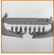
**6.** Turn all cuvettes **simultaneously** upside down, repeat several times
