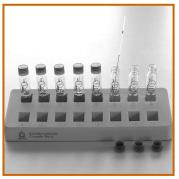
**1.** Eject all samples one after the other several times with micropipetter into cuvette
