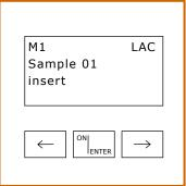
**3.** Switch photometer on with ON/ENTER key Wait for device check, confirm with ON/ENTER Select the required test, confirm with ON/ENTER
