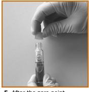
**5.** After the zero point adjustment of the last cuvette replace all screw caps with starter caps
