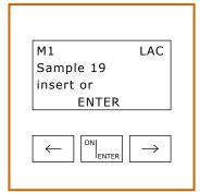
**4.** Zero point adjustment: Insert cuvettes with samples (Fig. 2) one after the other into photometer, all zero points are stored in memory
