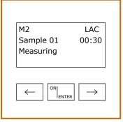
**7. First** press ON/ENTER key **Then** insert 1st cuvette into photometer
