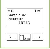
**5.** Zero point adjustment: Insert cuvette with sample (Fig. 3) into photometer, zero point is stored in memory
