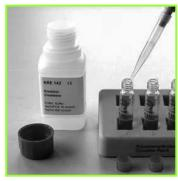
**1.** Pipette 1 mL buffer solution into each cuvette, then close cuvettes
