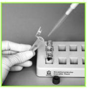
**3.** Transfer 500 µL of the sample (serum/plasma) into the cuvette
