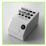
**4.** Incubate the cuvette with the sample for exactly 1 minute
