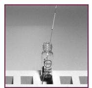
1. Insert capillary with 100  $\mu\text{L}$  sample (serum/plasma) into cuvette
