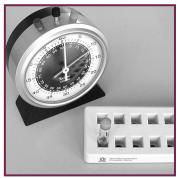
**4.** Leave the cuvette for 10 minutes at room temperature
