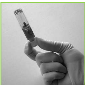
7. Turn cuvette upside down several times
