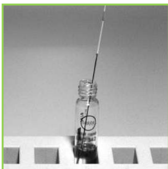
1. Insert capillary with 10 µL sample into cuvette
