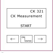
**5.** Switch photometer on with ON/ENTER key
