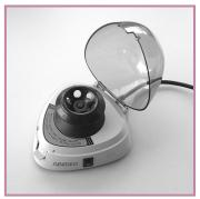
2. Insert reaction tube "R" with capillary into mini centrifuge Centrifugate for 1 minute
