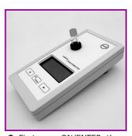
8. First press ON/ENTER, then insert cuvette into photometer Wait for measured value Compare the measured value with the target value on the package insert
