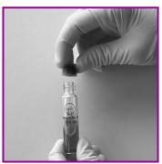
**2.** Screw the control cap onto a cuvette of the test you want to check
